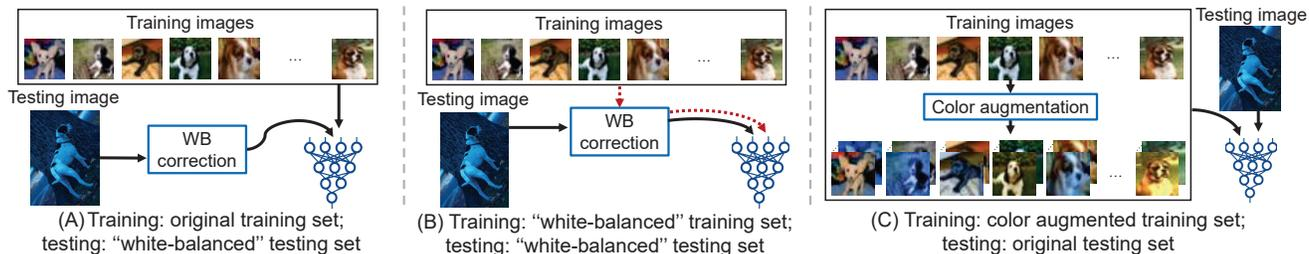
Figure S4. Different strategies to deal with improperly white-balanced images. (A) Traditional training process with unprocessed training set and applying a pre-processing WB correction step to each image in the inference phase. (B) Applying a pre-processing WB correction step to both training and testing images. (C) Color augmenting training images without any pre-processing applied during the inference phase. In (A) and (B), we used the WB-sRGB method [1] for the pre-processing WB correction.
